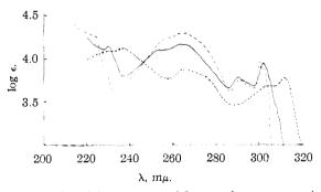
Fig. 2.—Ultraviolet spectrum of fluorene (— — — — ), 3-fluoro-6-methoxy-9-trifluoromethylfluorene (III, X = F) (|–| |–| |–| |–|) and 3-fluoro-6-acetoxy-9-trifluoromethylfluorene (— — ) in ethanol.
